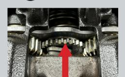
Webb heavy-duty NH225 and LN225 calipers are equipped with a robust centralized gear-driven adjuster, offering enhanced reliability and durability.
